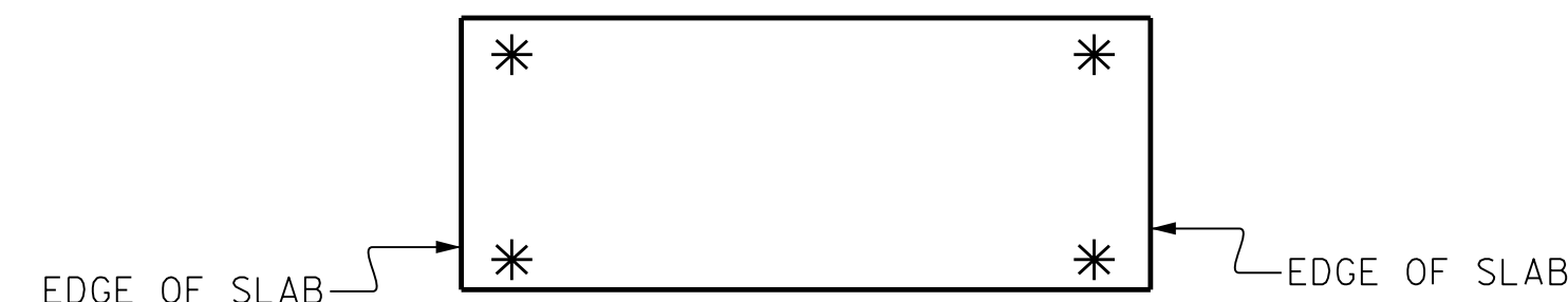
SKETCH SHOWING POINTS OF ATTACHMENT * DENOTES GUARDRAIL ANCHOR ASSEMBLY
